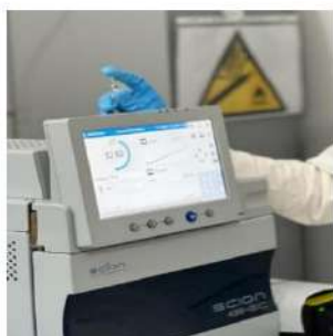
Figure 3. Capsicum annum extract injection in GC – FID in the laboratory.
