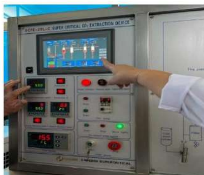
Figure 2. The Supercritical CO 2 extraction apparatus while performing in the laboratory.
